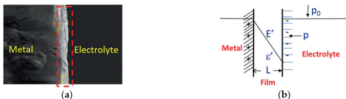
Figure 4. Interface between electrode surface and electrolyte: (a) SEM and (b) electrical double layer model of oxide film redrawn from [35]. Reproduced with permission from N. Sato, Vol. 16, 1683–1692, Electrochimica Acta; published by Elsevier, October 1971.
